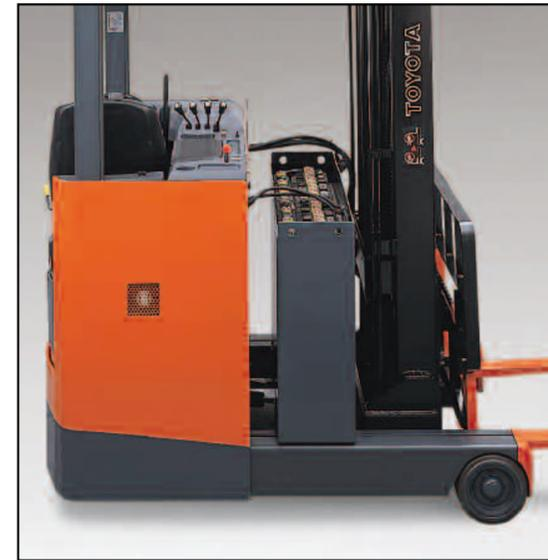
Other features, like the Power Battery Carriage encourage regular battery inspections, necessary for ensuring long service life.
