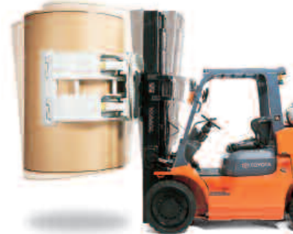
The Active Mast Function Controller controls the mast angle and speed depending on the weight and height of the load.
